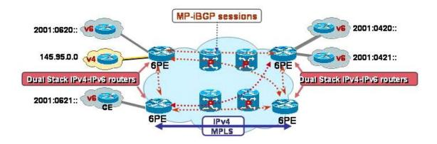
Figure 7: Example of a 6PE Topology within One AS
